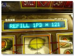
You can record the amount of coins you have refilled by a meter that is situated near the coin slot as shown here, then making a note of the numbers before and after you have refilled the machine, numbers shown in increments of 10p units
